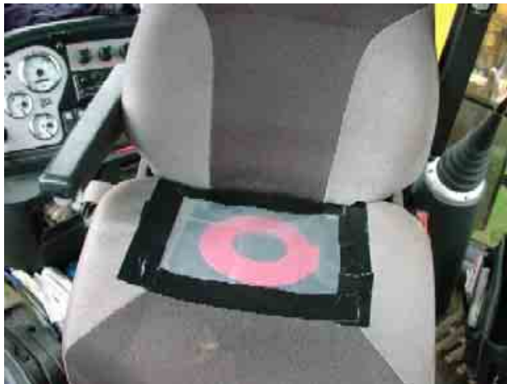
Figure 2.2 'Seat' accelerometer configuration incorporating operator presence switch
