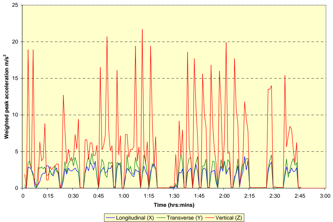
Figure A1.11.7 Linde 2.5 tonne fork lift truck:- time histories of weighted 1-minute peak seat accelerations (X, Y and Z-axes)
