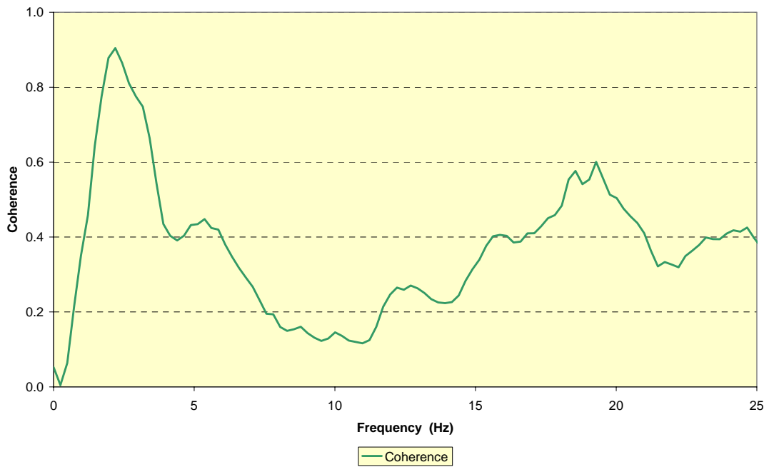
Figure A1.8.9 CAT 950F II articulated loading shovel:- seat transfer function – Coherence
