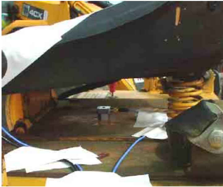
Figure 2.3 Tri-axial 'Floor' accelerometer installation using magnetic mounting
